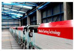
"In the photos, you can see the positioning of a grader Calistar (8 lines, 70 outputs): the beating heart of the plant. In particular, the detail of the fruit carriers: the grader clamps that makes the fruit travel upside down. It sounds bizarre, but it has its advantages: clean mechanical, electrical and electronic components, designed all above the floor, direct feeding from water, no transfers so extremely fruit friendly, and in addition it is incomparably quiet"
